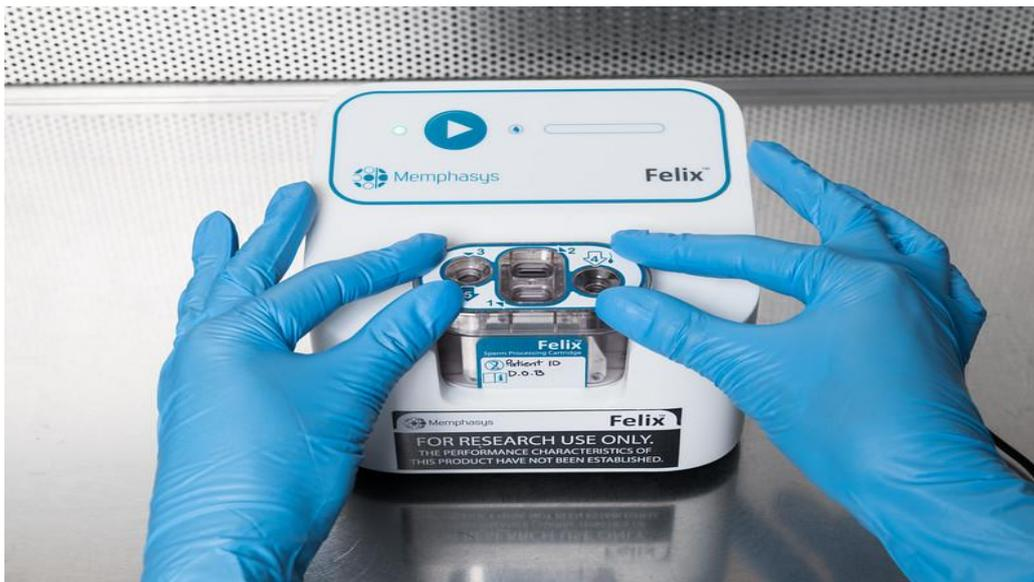
The Felix™ system separates high quality <sup>(1, 2)</sup> sperm from raw semen by a process combining electrophoresis and size exclusion membranes.
